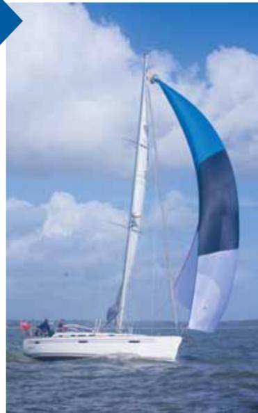
**ON A DEAD RUN:** As we saw last month, the chute becomes blanketed by the mainsail as the boat approaches a run. That's just what you want when hoisting and dropping, but not when you're trying to keep it driving. The tendency to become blanketed is perhaps the greatest weakness of a cruising chute flown in the conventional manner.
