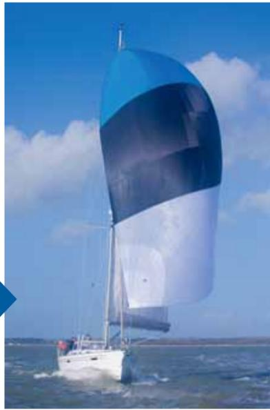
**SAILING CLOSER:** To sail closer to the wind, tension the tack line to take some of the curve out of the luff, and sheet in. Here the apparent wind is at about 90° – pretty well on the beam. That's good going for this wind strength: a combination of a well-cut sail and a well-behaved boat. In lighter conditions it could be used closer than this.
