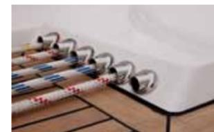
Control lines led aft from the mast run through the moulding that forms the hatch garage
